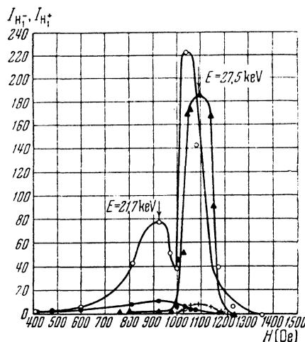
FIG. 1.  $\blacktriangle$  — positive ion current obtained without a foil (the scale is reduced 200 times);  $+$  — negative ion current obtained without a foil;  $\circ$  — positive ion current, with foil in place;  $\bullet$  — negative ion current, with foil in place.
