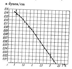
for all three capillaries, are shown in the figure. At very low temperatures, the mean error of measurement amounted to  $\pm 5\%$ , with the maximum error  $\pm 7\%$  The maximum spread of the individual measurements is shown by the arrow on the graph.
